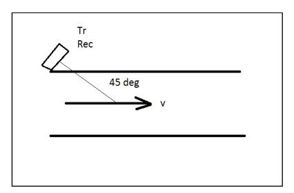
Diameter= 2cm => Radius= 1cm = 0.01m Area=  $\pi$  r<sup>2</sup> = 3.14 x 0.01 x 0.01 = 3.14 x 10<sup>-4</sup> m2 Frequency = 40kHz  $V_p = F_0 \lambda$  $\lambda = 331/40000 = 8.275mm$  $|Kr|cos45 = |Ki|cos45 = 2 \pi/\lambda x cos45 = 536.632$
